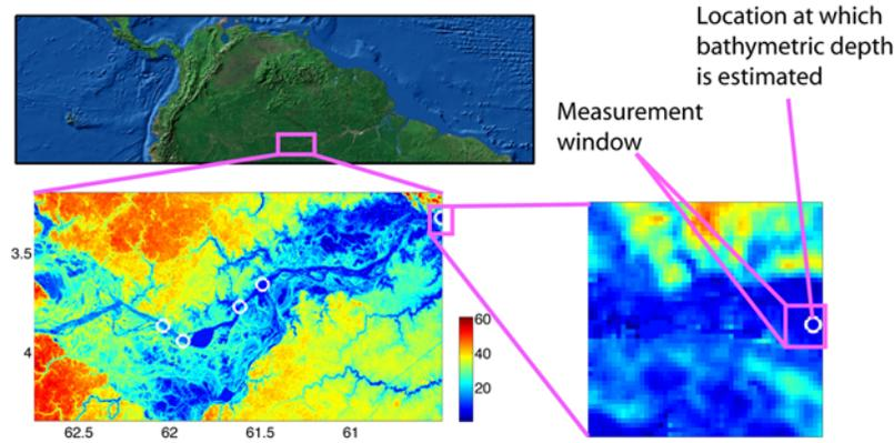
**Figure 1.** (bottom left) The study area DEM in (top) the Amazon River basin is shown. The white circles are the locations at which channel depth is estimated. (bottom right) Channel depth is estimated using SWOT floodplain WSE measurements in the measurement window, illustrated for the far downstream location.
