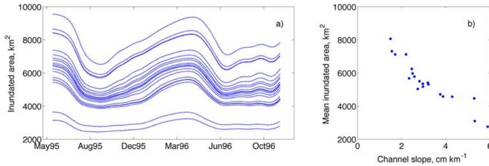
**Figure 2.** (a) Inundated area output from the LISFLOOD-FP model is shown for the 22-month study period for the ensemble of model runs. (b) The relationship between the bathymetric slope and temporal mean inundated area is also shown.
