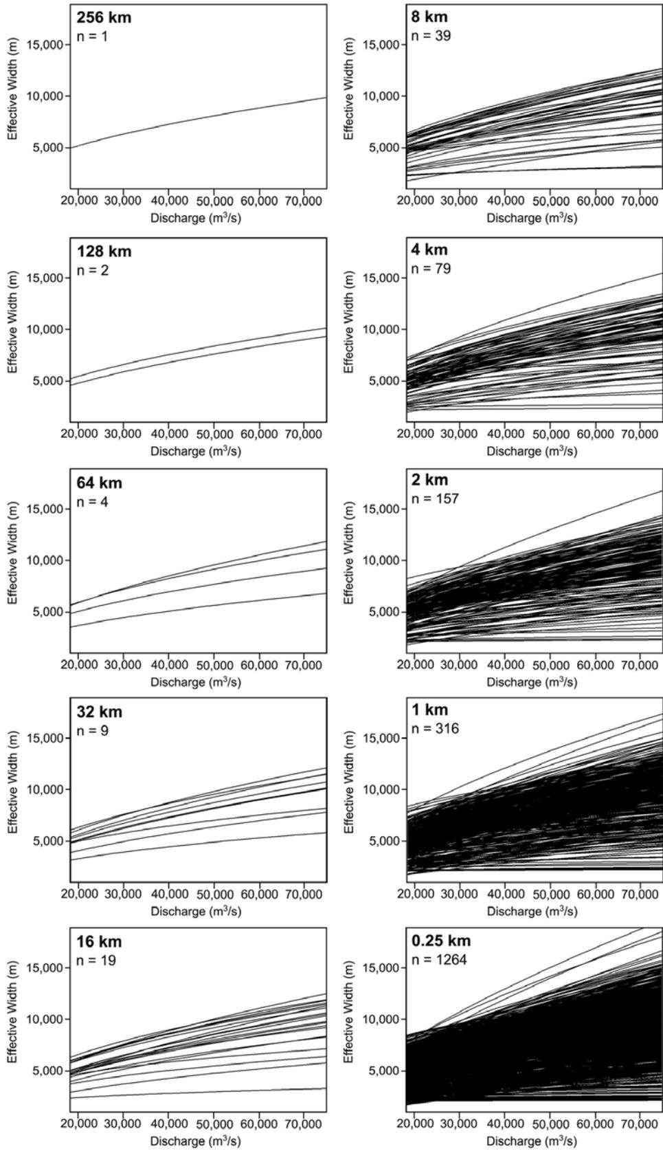
**Figure 4.** Distribution of best fit  $W_e - Q$  rating curves for 10 example reach length scales. Each rating curve is obtained from a different location along the river. Rating curves from different river reaches display increasing similarity as reach length is increased.
