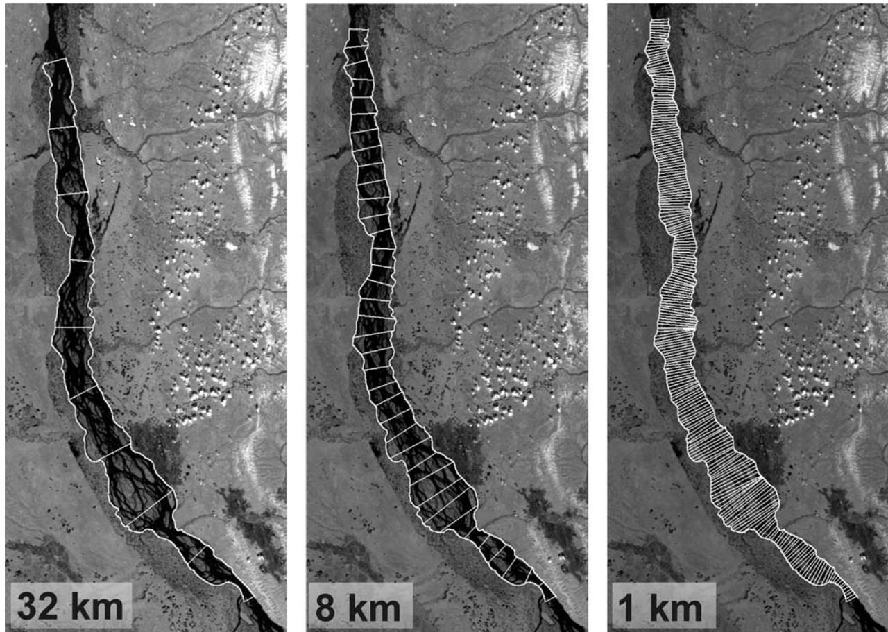
**Figure 2.** Sample MODIS image of the large braided reach used in this study, illustrating disaggregations of 32, 8, and 1 km reach length scales. Water surfaces appear dark, and white objects are clouds.
