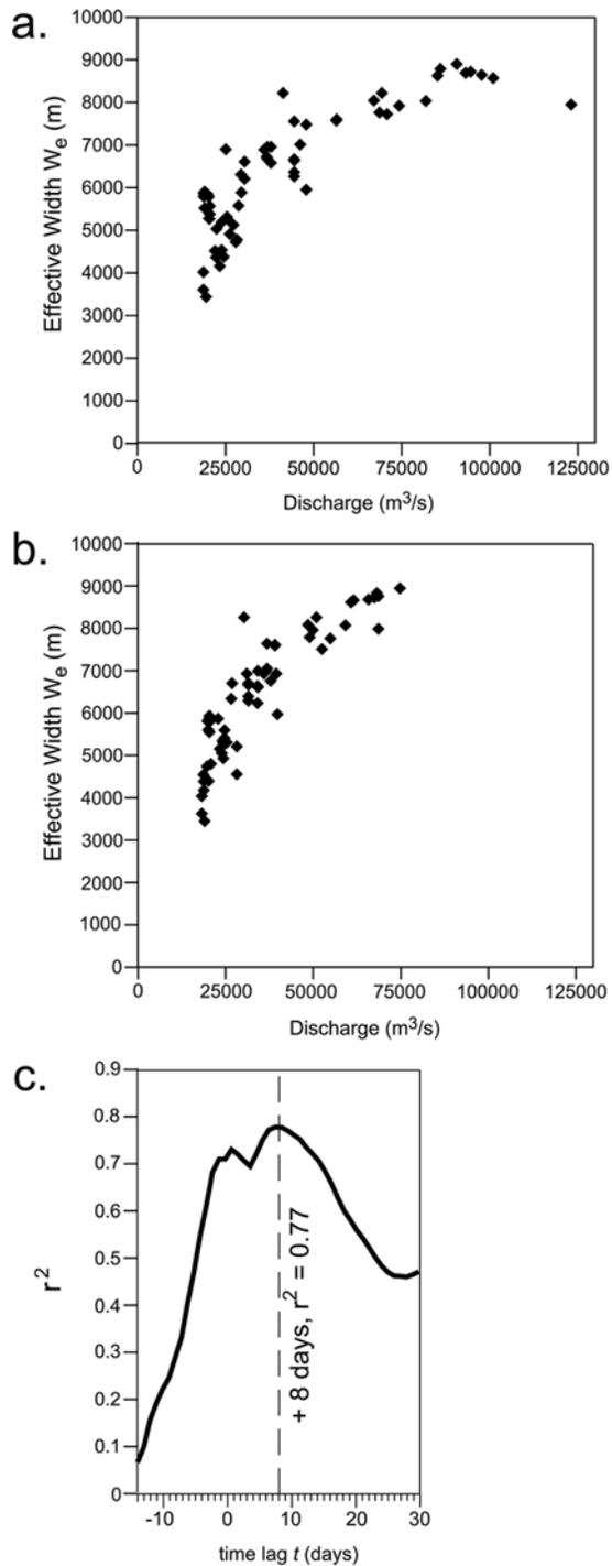
**Figure 3.** (a) A power law relationship is found between satellite-derived effective widths ( $W_e$ ) and same-day ground measurements of river discharge ( $Q$ ). (b) However,  $W_e - Q$  rating curve scatter decreases when a time lag is introduced between the two variables. (c) Maximum correlation is achieved by lagging observed  $Q$  8 d behind satellite-derived  $W_e$ , obtained  $\sim 700$  km upstream.
