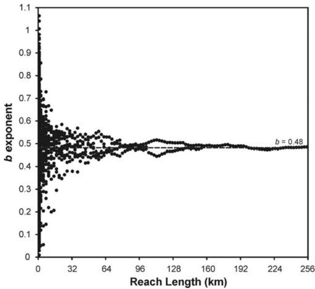
**Figure 5.** Distribution of  $b$  exponents for the full spectrum of reach length scales examined in this study (0.25–256 km). Convergence to a stable value ( $b = 0.48$ ) is achieved at length scales  $> \sim 60$ – $90$  km (2–3 times floodplain valley width).
