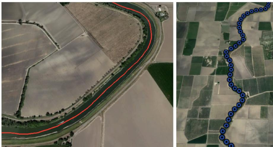
**Figure 2.** [Left] Aerial view of a river with SWOT centerline in red. [Right] Blue circles show example *node locations* defined at fixed intervals along the centerline. See text for more details. **Image credit:** Michael Durand [Ohio State University]
