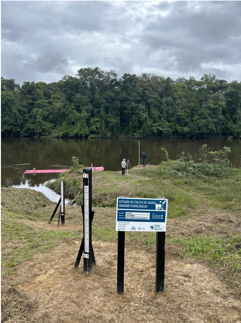
Figure 2. Visit to Water Level Gauge Stations to GNSS levelling and data collection. (Credits:SGB/CPRM).
