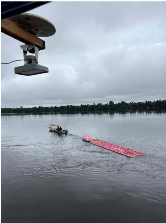
Figure GNSS CALNAGEO and GNSS + RADAR on boat to mapping water level surface. (Credits:SGB/CPRM).
