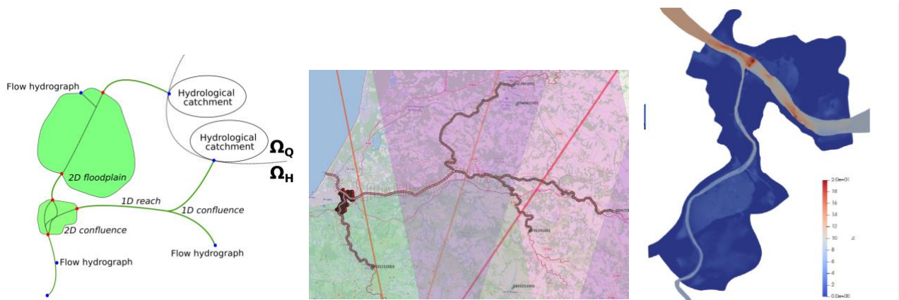
Fig. 9 from [PuGaMoetal21a,b]. (Left) Schematic representation of the multi-D hydrological-hydraulic model. (middle) basin hydrological-hydraulic mesh: spatially distributed hydrological modeling for lateral/upstream inflows, 1D like river network with mesh based on bankfull water extents internally coupled to fine 2D zooms (ex. floodplains, confluences), (right) zoom on the flow depths simulated around the city of Bayonne with the multi-D chain (data courtesy: flood forecasting center SPC-GAD, INRAE).
