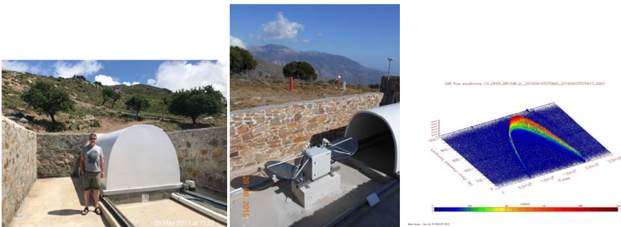
Figure 3. Upper right: ground tracks of SWOT Pass No.58 (light blue), Jason (red), Sentinel-3A (green) and Sentinel-3B (blue) missions over the CDN1 transponder Cal/Val site. Lower: The microwave transponder at the CDN1 Cal/Val site and the transponder response on the CryoSat-2.
