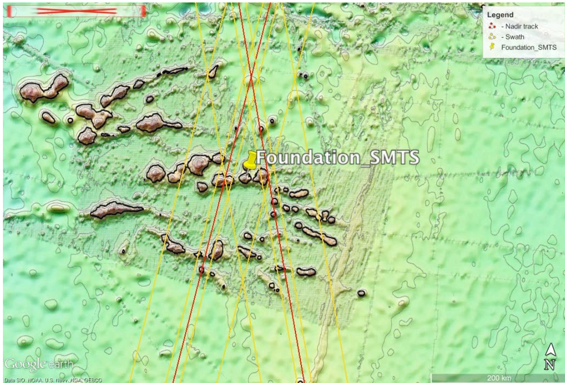
Figure 4. High-resolution (500 m) bathymetry of the Foundation Seamounts in the South Pacific from extensive multibeam surveys of the R/V Sonne and R/V L' Atalante [Devey et al. , 1977]. Also shown are the swaths of the SWOT altimeter during the commissioning phase of the mission. Many of these large seamounts have crests shallower than 1000 m so produce high amplitude, high-resolution geoid slopes. This is also an region of low significant wave height and low mesoscale variability so it is optimal for exploring the ultimate resolution of the SWOT altimetry.
