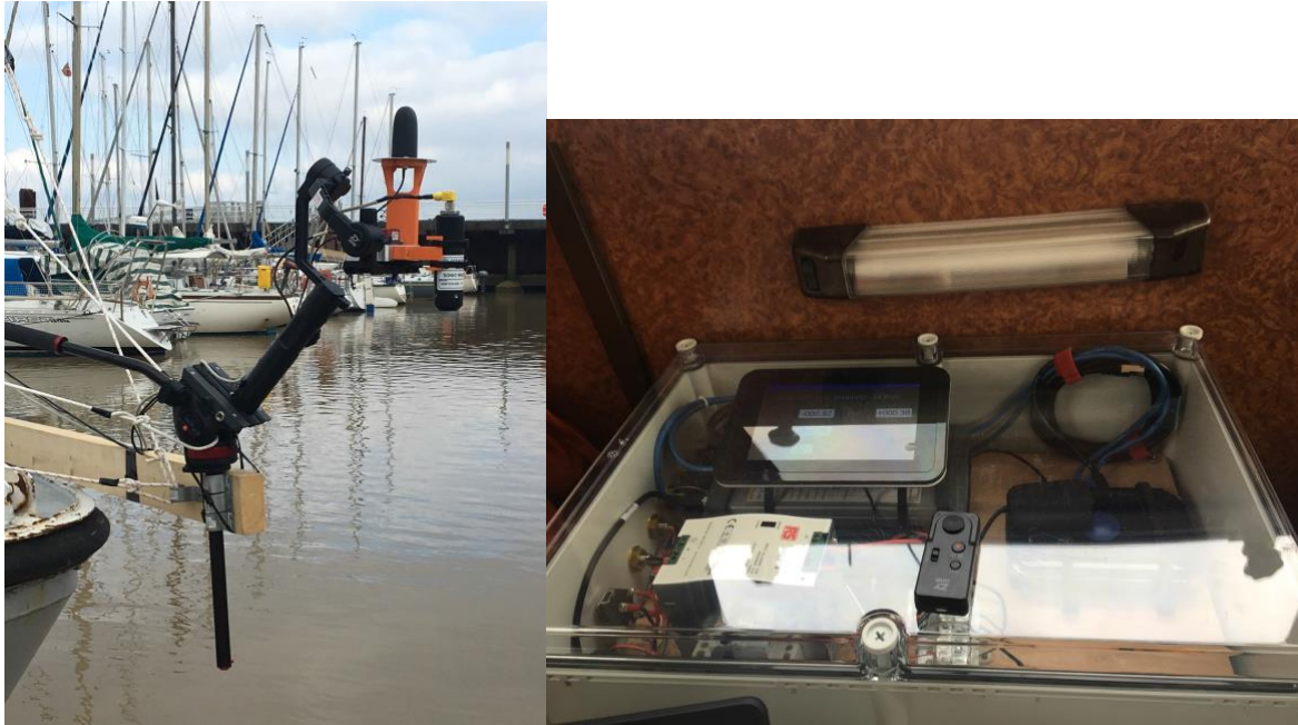
Figure 6. Left: photo of the system called "Cyclopee" (acoustic radar and GPS antenna mounted on a stabilizer arm) at the front of the boat during the campaign on the Gironde in October 2018. Right: photo of the electronic box containing the data acquisition and control/visualization system.
