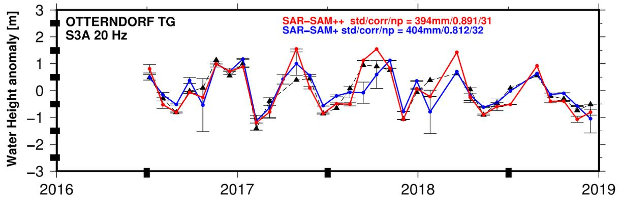
Figure 4. Time-series of water level from altimeter and in-situ corrected for the ocean tide.
