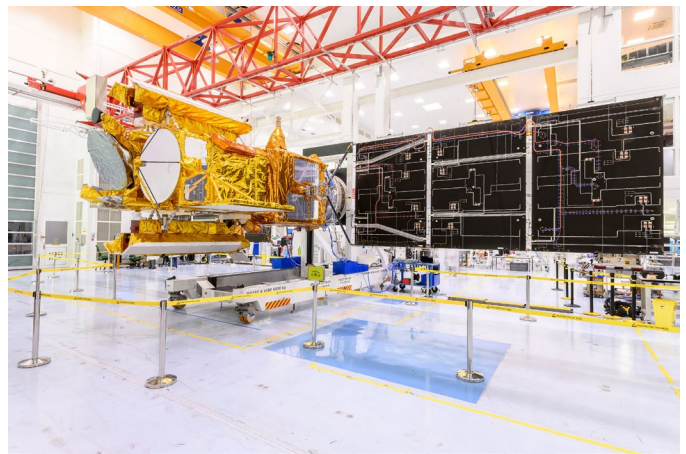
Engineers successfully deployed one of two solar arrays installed on the SWOT satellite in January 2022 at the Thales Alenia Space clean room facility near Cannes, France. Courtesy: CNES/Thales Alenia Space
