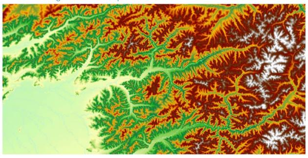
Example DEM from which a polygon shapefile of the river network can be derived.
