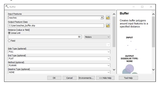
Distance can be specified using either a width field (if your polyline includes this attribute) or simply a constant linear value (e.g., 50 meters). Note that the distance is one-sided, meaning that to set a value of 50 meters results in a polygon width of 100 meters. A comparison between the polygon river reaches (black outline) and polyline river reaches (blue lines) is shown below. Once you have created the polygon shapefile, continue with the steps in Section 3A.
